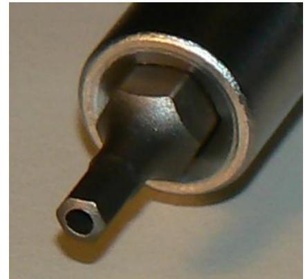
For the cover screws size 1/8 inch is required. For the removal of the harddisk size 2 mm is needed.
