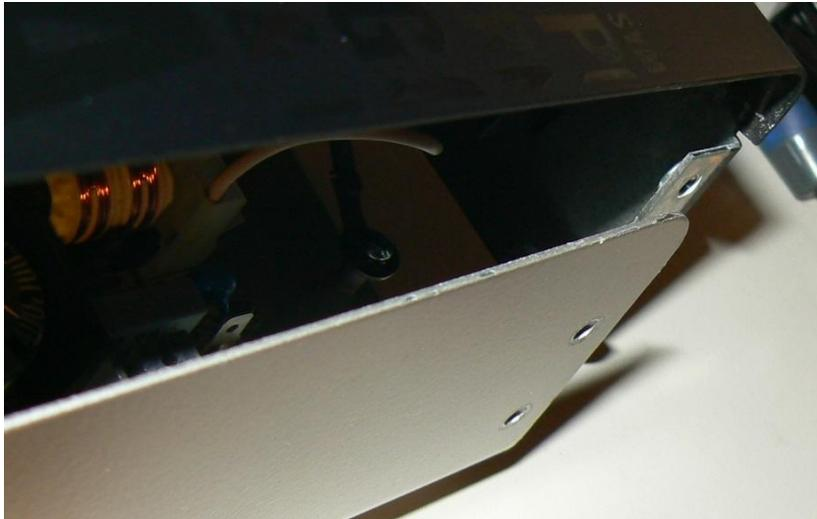
On the back, a connector to the power supply and the ground connection via a bolt to the chassis needs to be removed.
